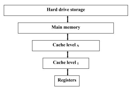
Figure 2.4: Memory hierarchy in current computing systems
