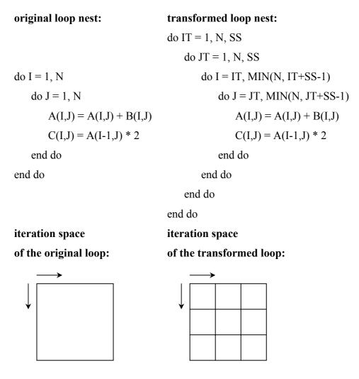
Figure 3.3: Loop tiling example
