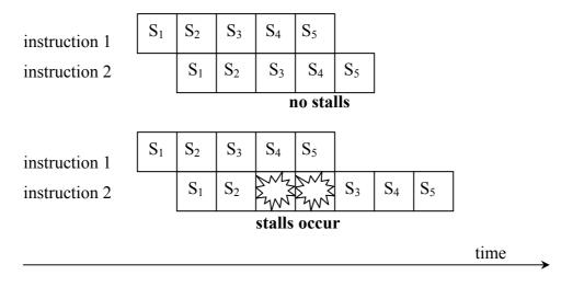
Figure 2.3: Instruction execution on a pipeline when stall occurs
