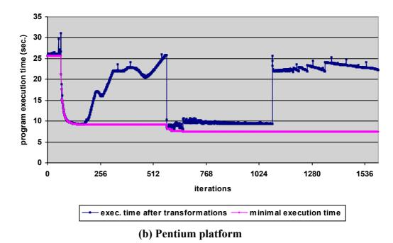
Figure 4.12: Changes in execution time during each iterative step (matmul)
