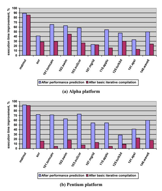
Figure 5.7: Overall potential and iterative performance improvement (%)
