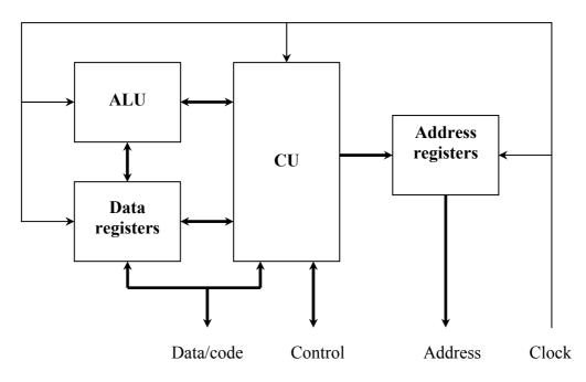
Figure 2.1: Von Neumann processor architecture
