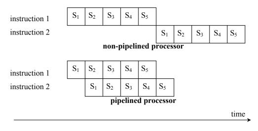
Figure 2.2: Instruction execution on non-pipelined and pipelined processors
